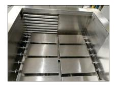
Immersible transducers are placed whenever you need in your existing tanks. These units gives you complete freedom to design specialized cleaning setup. (Upgrade pre soak tank with Ultrasonic Immersible transducers)
